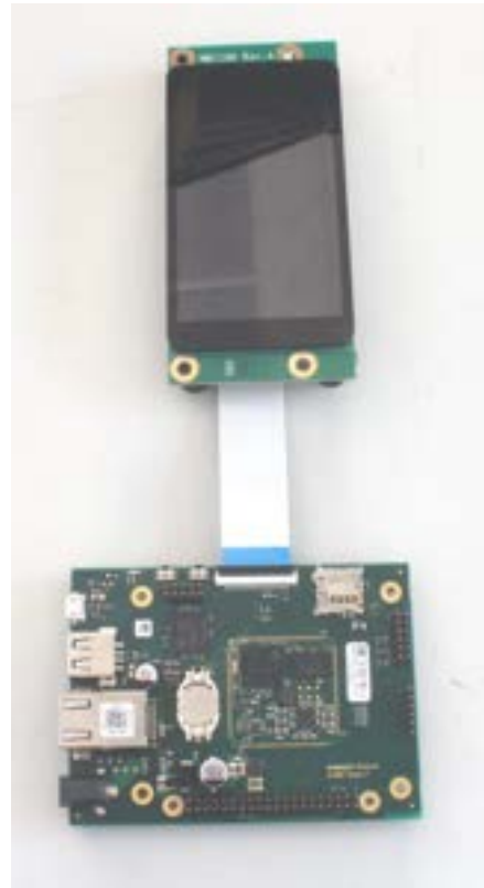
Connecting the B-LCD40-DSI Display (STMicroelectronics) via the DSI-adapter board
