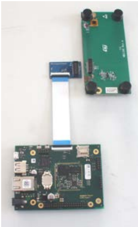
Connecting the B-LCD40-DSI Display (STMicroelectronics) via the DSI-adapter board
